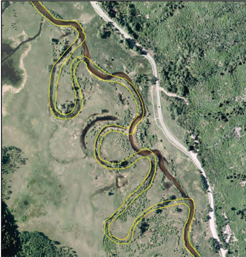
North Star's channel geometry observed in 1898, overlain on a modern aerial photograph. Golder Associates
