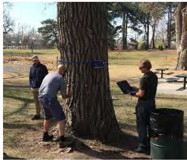
Figure 7. Tomograph measurements being taken on a tree in Washington Park, Denver, CO.
